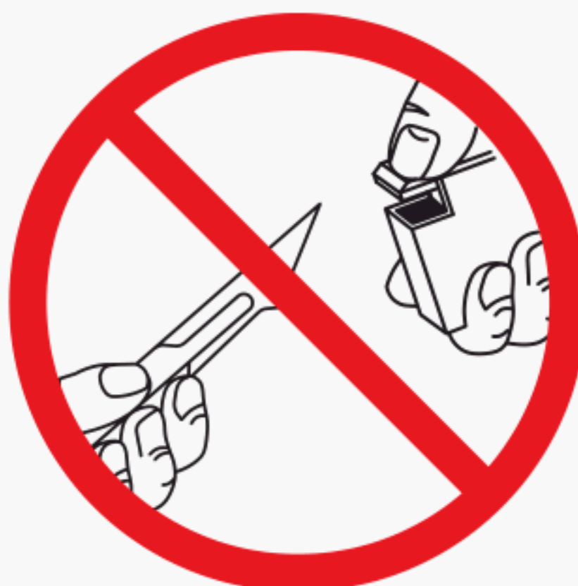
Figure 3 — Do not remove the scalpel blade using a resheathing-type removal action involving the use of both hands
