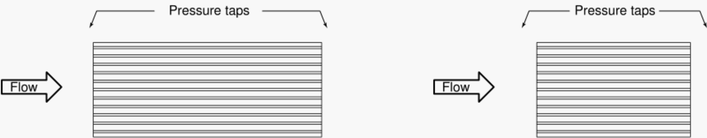
Figure 12—Laminar Flow Element
