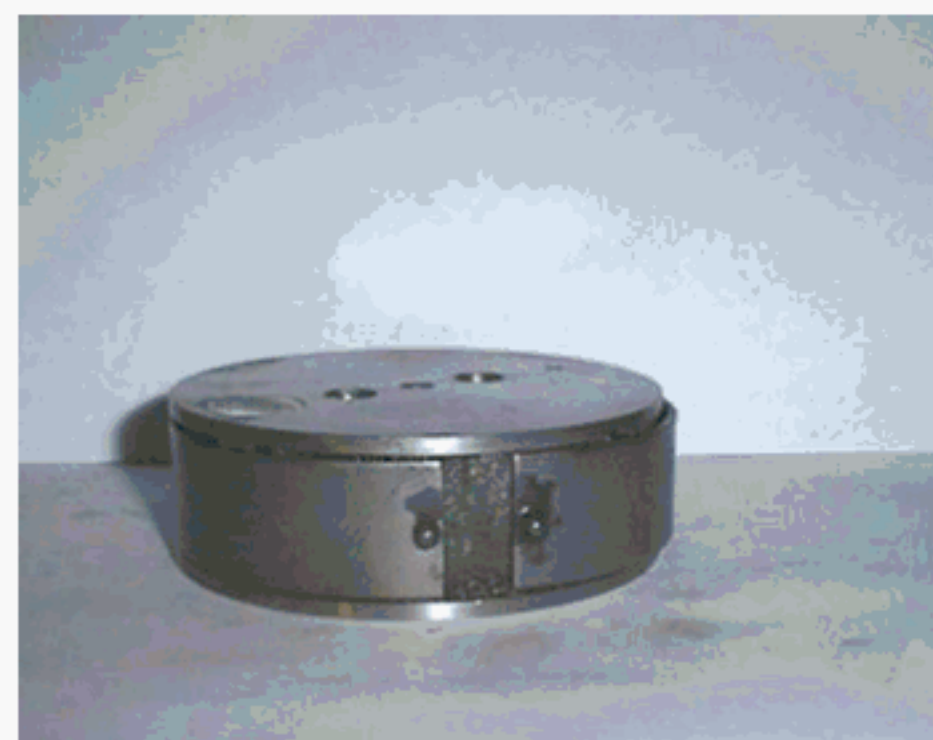
Figure 2 — Typical mould assembly (side view)
