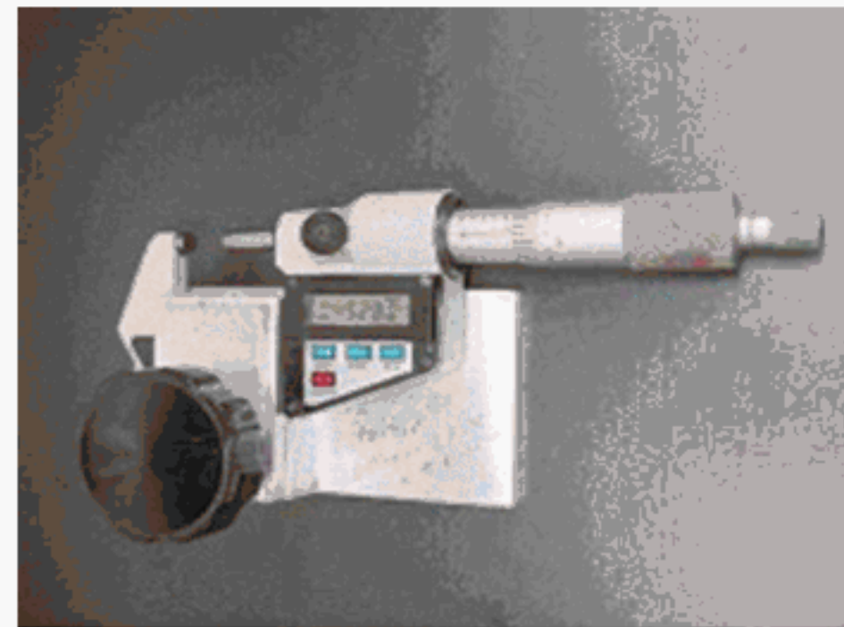
Figure 8 — Micrometer mounted to adapter
