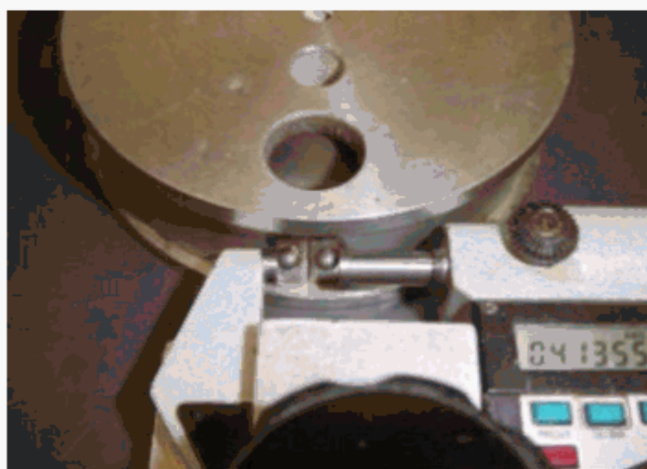
Figure 9 — Micrometer measuring
